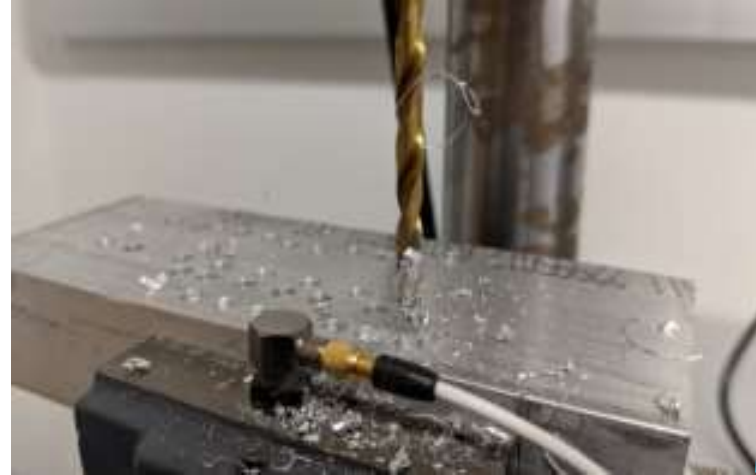
Accelerometer installed on the drilling vice
